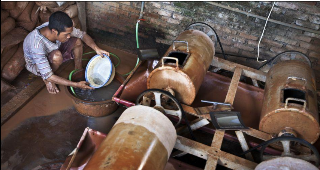
Figure 8. Water mixed with 400-500 gram of mercury is transferred to a bucket after being processed in the cylinder-shaped rock-crushing machines.
