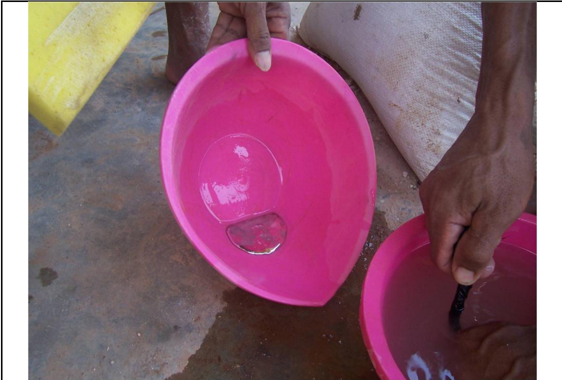
Figure 5. About 500 gram mercury added to each ball-mill and mixed for 5 hours. At the end of the process, the amalgam formed and bring to the gold shop to be burned. Photo: Yuyun Ismawati/BaliFokus.
