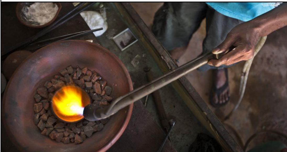
Figure 10. Workers burn the crushed ore, which has been mixed with mercury, hoping to capture flecks of gold. Mercury vapor would last in the air for 1-1,5 years.
