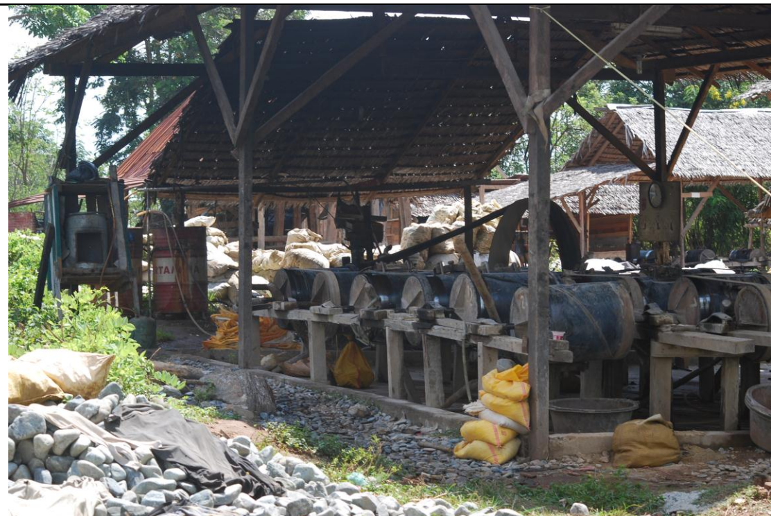
Figure 4. When the gold price was peaking up, more than 20,000 units of ball-mills were working 24 hours. Less than 20 plants obtained the business permits and the Environmental Impact Assessment reports from the Environmental Agency of Palu City. In June 2011, mercury vapor in this area measured as high as 45,000 ng/m 3 . Photo: Yuyun Ismawati/BaliFokus.
